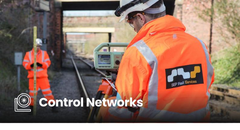
All projects, regardless of size or complexity, require the development of a reliable control grid to guarantee that all design and construction works relate to the same coordinate system.
