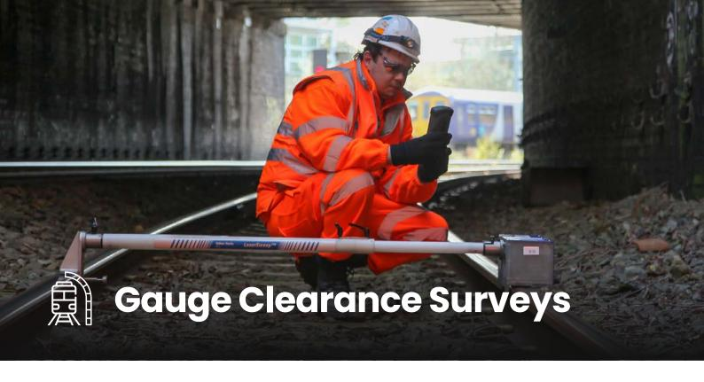
Working to Network Rail Standard NR/L2/TRK/3203 and supported by our sister firm, SEP Rail Design, we use cutting-edge laser measurement equipment and software to deliver the profile and clearance information your projects so desperately need.
